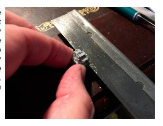
If all your cuts were parallel, the bottom of the carb will be completely flat except for a little nub in the middle. Use a knife or sandpaper to remove that nub and make the bottom completely flat. Congratulations, your scale carburetor is now ready to be painted and installed on your engine! Be careful with all the little details that stick out from the carb; resin is pretty strong but they can be snapped off if not handled carefully.
